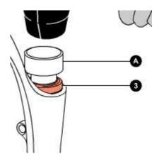
Using a small flat-tip screwdriver, fit the stop ring (2) and check that it fits perfectly into its groove. Take great care not to damage the internal surfaces of the one-piece assembly when fitting the stop ring.
