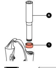
Using a hammer knock the introducer (A) into the arch-slider assembly.
