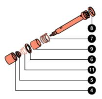
If the piston segment (8) is damaged, you can prize it off with a small flat-tip screwdriver.
