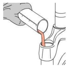
A lower or higher volume or a type of oil other than the one recommended can change the behaviour of the fork in every phase.
