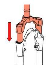
In a graduated recipient, prepare the quantity of oil to pour into the fork leg (see table). Pour roughly 1/3 of the oil required into each stanchion, then pump the fork a few times to eliminate any traces of air.
