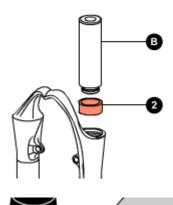
Using a hammer knock the introducer  $(\boldsymbol{B})$  into the arch-slider assembly.
