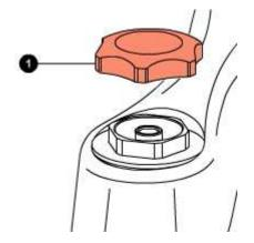
Using a small pin screwdriver, blow the air off the fork leg, pushing on the air valve. Fully unscrew lock cap (2) with a 21mm socket spanner. Remove lock cap (2).
