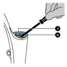
The old sealing rings and dust seals must not be used again.
