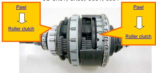
Roller clutches are used in place of pawls in two places to reduce noise. The new hubs are now almost completely silent, there is only a ratcheting noise when backpedaling.
