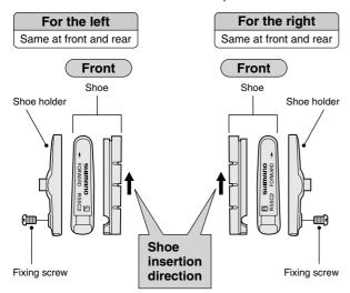
4. Tighten the fixing screw.
