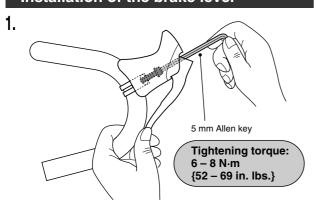
In the case of carbon handlebars, it may be necessary to lower the tightening torque in order to prevent damage to the handlebar. Please consult the bicycle or handlebar manufacturer regarding the appropriate level of tightening torque for carbon handlebars.
