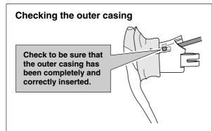
**3.** Temporarily secure the outer casing to the handlebar (by using tape or similar material).
