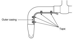
4. Then wrap the handlebar with handlebar tape.
