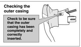
**3.** Temporarily secure the outer casing to the handlebar (by using tape or similar material).
