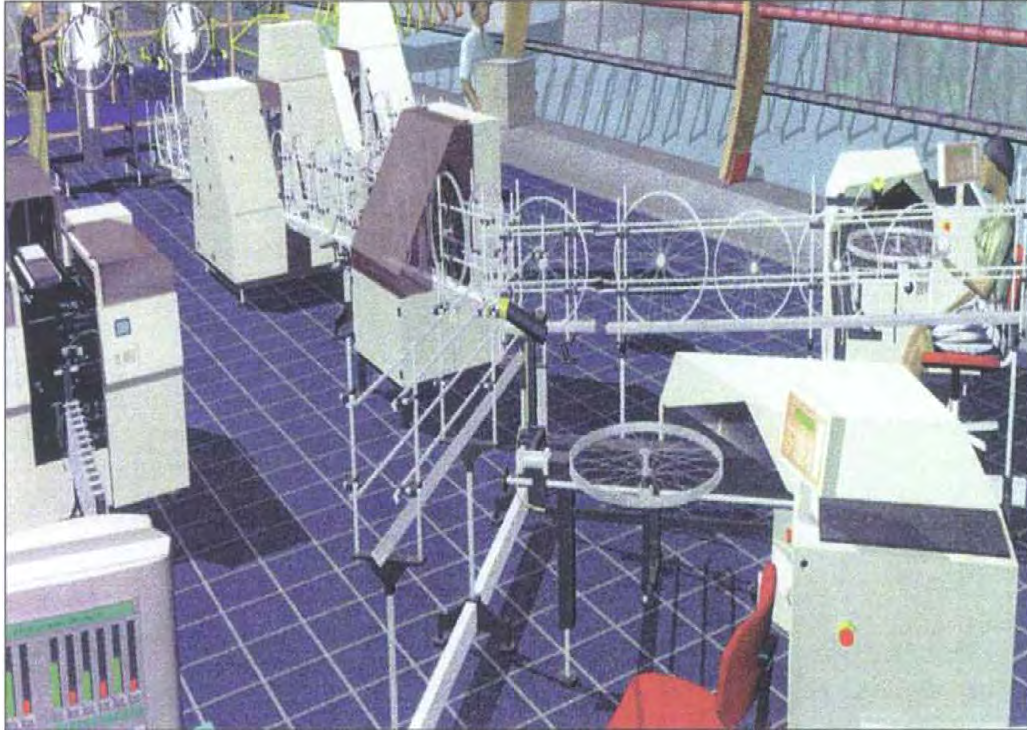
Layout of □ central controlled truing facility. (HOLLAND MECHANICS)
