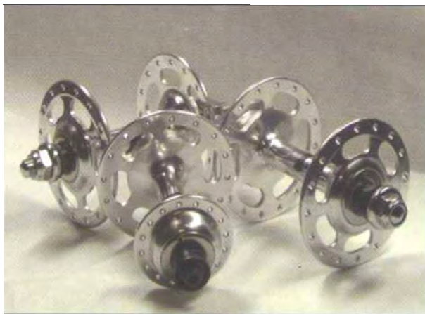
High flange hubs, the one in the center is a "hi•low" hybrid, produced once by Campagnolo and called "Piccolo-Grande".
