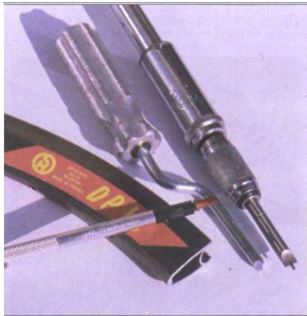
Spoking tool, from left nipple holder ULLMANN DEVICES, nipple driver BICYCLE RESEARCH, hand drill VAR with bit.
